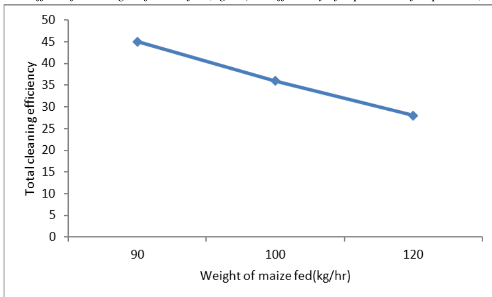
Figure 16: Effect of the weight of maize fed (kg/hr.) on total cleaning efficiency
