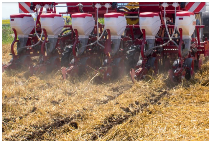
Figure 1: Sowing unit of direct drill machine
