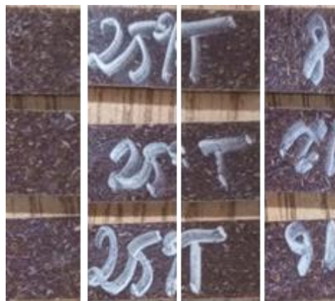
Figure 3: Samples cut to monitor the evolution of composite residual mass as a function of temperature.
