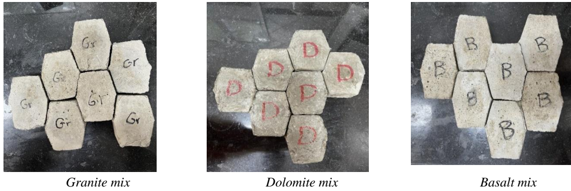
Figure 1: The produced hexagonal paving unit from different aggregate mixes.
