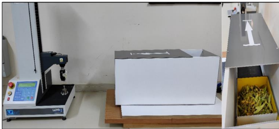
Figure 2. The mechanism used for determining frictional properties
