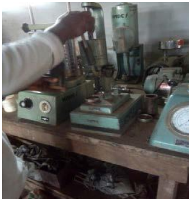
Figure 7: Sand rammer for making sand test sample
