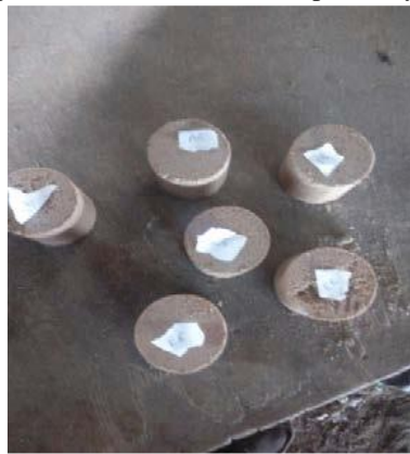
Figure 4: Sand test samples for permeability test
