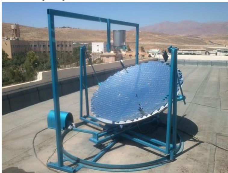
Figure 6: Photograph of the concentrator used to dry calcium hydroxide.
