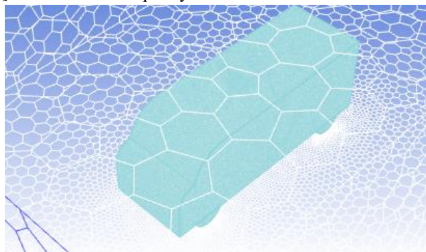
Figure 5: Polyhedral mesh for vehicle speed v = 40 \text{ km/h} and closed window.
