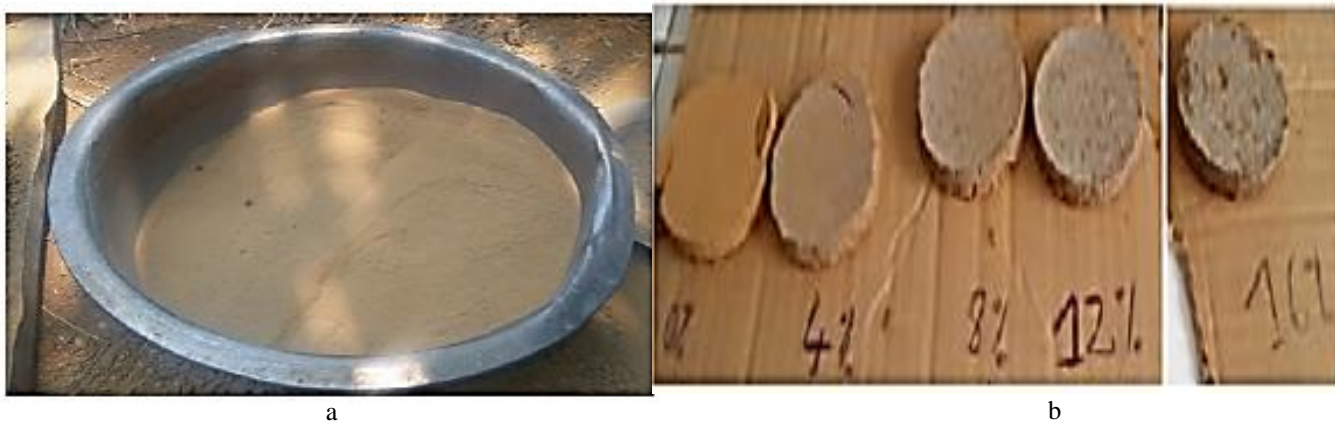
Figure 7: (a) Dry soil powder obtained with a 0.4 mm sieve, intended for the preparation of patties. (b) Dry clay patty, stabilized with molasses, after one week of drying.
