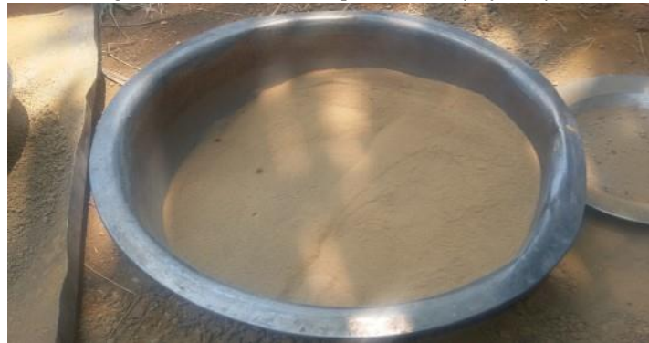
Figure 4: Powder of obtained soil from sieve 0.4mm, intended to the preparation of stabilized clay cakes
