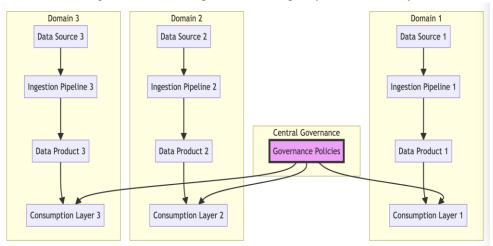
This diagram illustrates the decentralized data ingestion and processing architecture within a Data Mesh. Each domain is responsible for ingesting data from relevant sources and transforming it into consumable data products, while a central governance layer ensures compliance and standards across domains.
