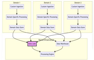
This diagram shows the self-serve data infrastructure where shared components like data lakes and data warehouses support domain-specific ingestion, processing, and storage. Each domain customizes its infrastructure needs while leveraging shared resources for efficiency and scalability.
