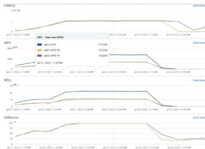
Figure 3: Maximum storage IO capacity with 70:30 Read:Write Ratio
