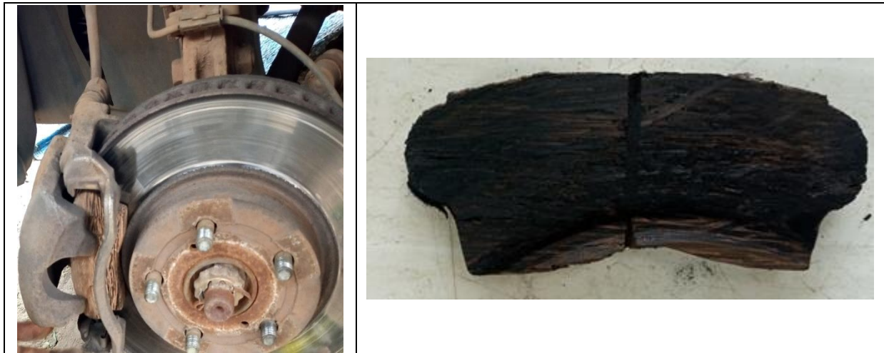
Figure 4: Pad tested on a car wheel
