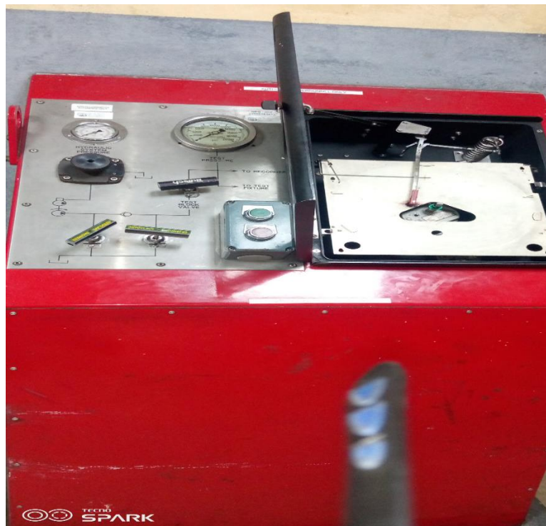
Figure 4 Pressure test chart recording unit.
