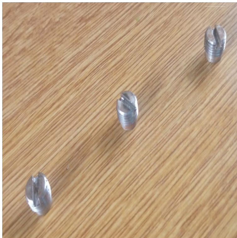
Figure 5: Sample of steel shear screws for smart well completions pressure sensitive hydro tip nipple sub
