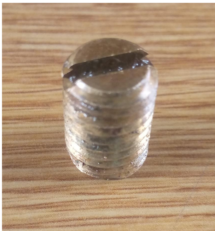
Figure 6: Sample of brass shear screws for smart well completions pressure sensitive hydro tip nipple sub
