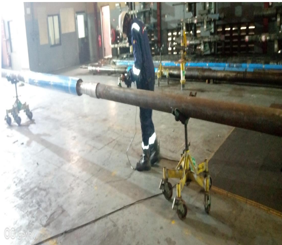
Figure 2: Buffing was carried out to remove minor scales and rust from the transition pup joints on the packer assembly.
