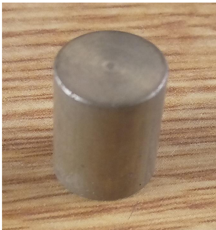
Figure 7: Sample of brass shear pin for smart well completions pressure sensitive hydro tip nipple sub
