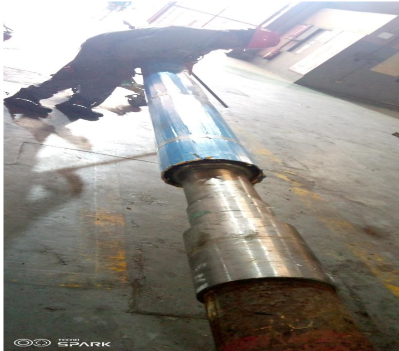
Figure 3 The packer elements and main body was wrapped with lamiflex to protect the sensitive elements
