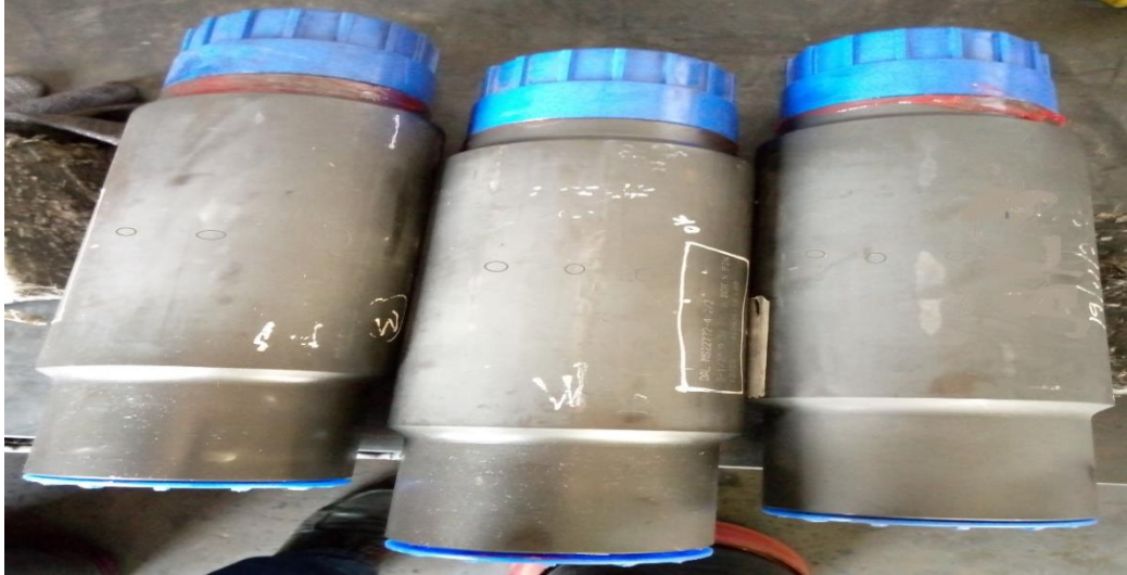
Figure 8: Sample of smart well completions pressure sensitive hydro tip nipple sub
