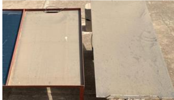
Figure 2: Test platform (CIGS on the left and CdTe/CdS on the right)
