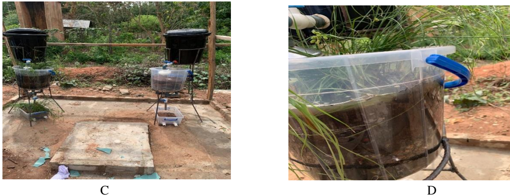
Plate 2: Image (c & d) Complete set up (vegetative/non vegetative filters) for domestic wastewater treatment unit and macrophyte inclusion in wastewater filtration system.
