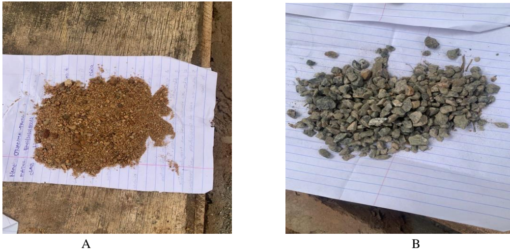
Plate 1: Image (a & b) Soil and gravel filters for domestic wastewater treatment
