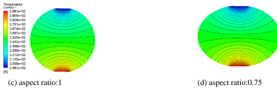
Fig. 5 Temperature distribution of longitudinal section of particles with different aspect ratios under adiabatic condition
