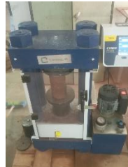
Figure 6: Determination of compressive strength
