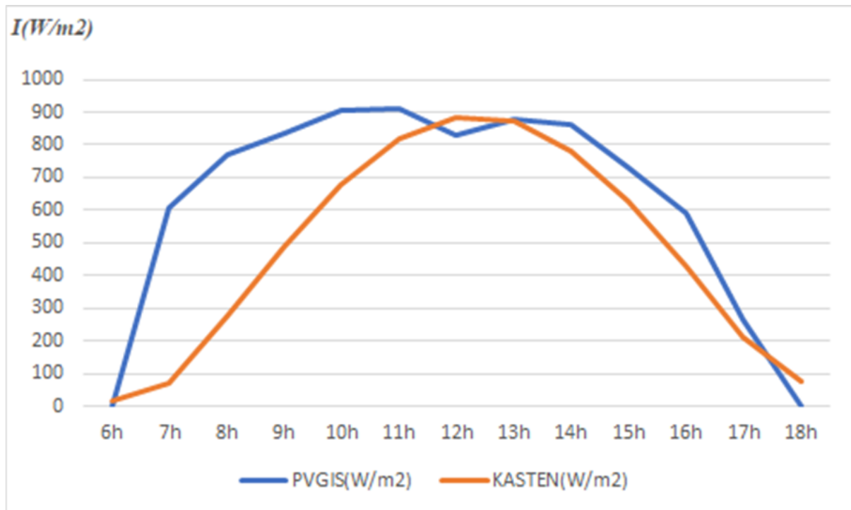
Figure 4: Curve of the evolution of the irradiation of the day in February
