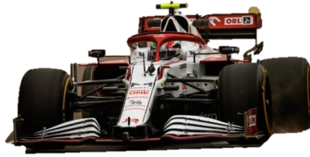
Figure 17: Alfa Romeo's C 39 2021 F1 vehicle produced by additive manufacturing of more than 300 parts [28].
