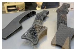
Figure 13: F1 Brake pedal designed for the 2016 Redbull Formula 1 car (Photo by Michael Petch) [22].
