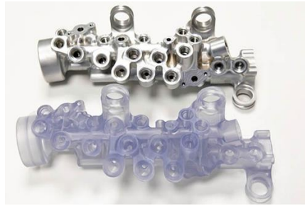
Figure 19: A hydraulic manifold produced with CNC machining (at the top) and with SLA (at the bottom) (below) by the Renault F1[18].
