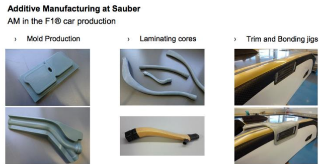
Figure 11: Pictures of molds, lamination cores, trim and bonding gauges made by additive manufacturing [28].
