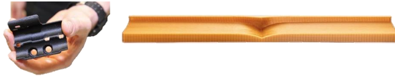
Figure 14: The McLaren Formula 1 team's MCL32 race car a. bracket b. rear wing [31].
