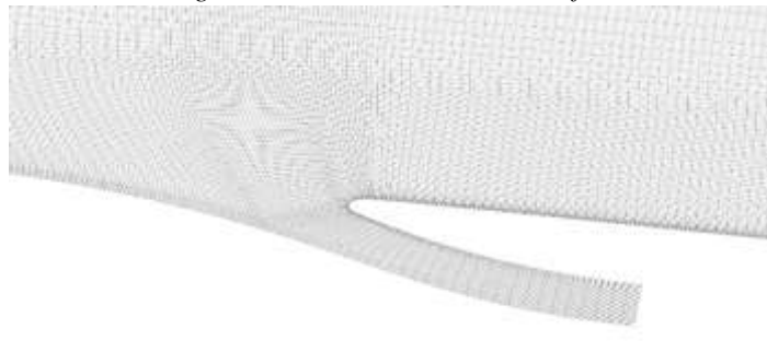
Figure 2: Suction device mesh (extrados)
