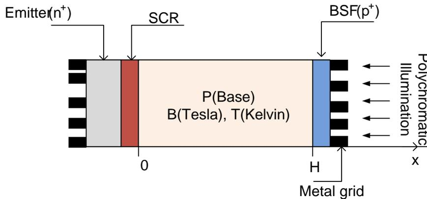
Figure 1: Back side illuminated  $n^+ - p - p^+$  silicon Solar cell, under both the magnetic field and the temperature
