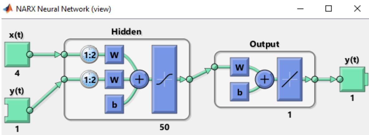
Figure 2: Model architecture in the View of the Network window
