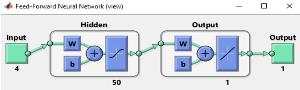
Figure 1: Synoptic diagram of the architecture of MLP neural network models with 50 neurons under the hidden layer
