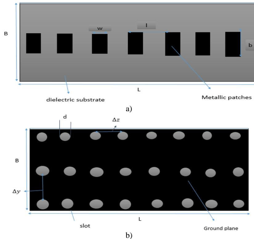
Figure 1: A defected ground plane microstrip leaky-wave antenna a) Top view; b) Bottom view (defected ground plane)
