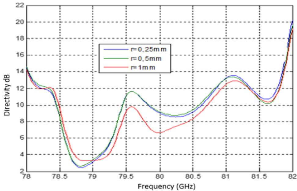
Figure 3: Directivity of the defected ground plane microstrip leaky-wave antenna  $b=0.8\lambda_0$  ;  $l=2.5mm$  ;  $w=0.3387\lambda_0$  ;  $B=8\lambda_0$  ;  $\Delta y = \Delta z = 1.0667\lambda_0$  ;  $N=11$
