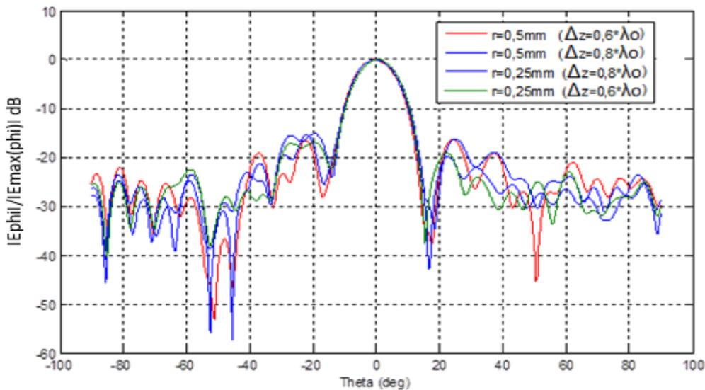
Figure 5: Radiation patterns of the E-plane at  $F=80$  GHz,  $b=0.8\lambda_0$  ;  $l=2.5$  mm ;  $w=0.3387\lambda_0$  ;  $B=8\lambda_0$  ;  $\Delta y=1.0667\lambda_0$
