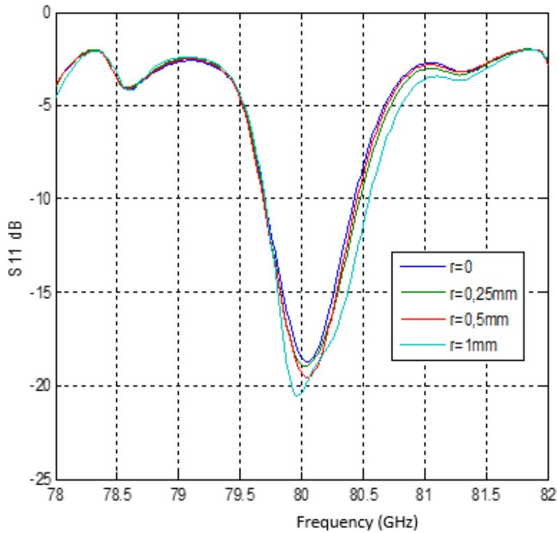
Figure 2: Reflection coefficient of a defected ground plane microstrip leaky-wave antenna  $b=0.8\lambda_0$  ;  $N=11$  ;  $l=2.5mm$  ;  $w=0.3387\lambda_0$  ;  $B=8\lambda_0$  ;  $\Delta y = \Delta z = 1.0667\lambda_0$
