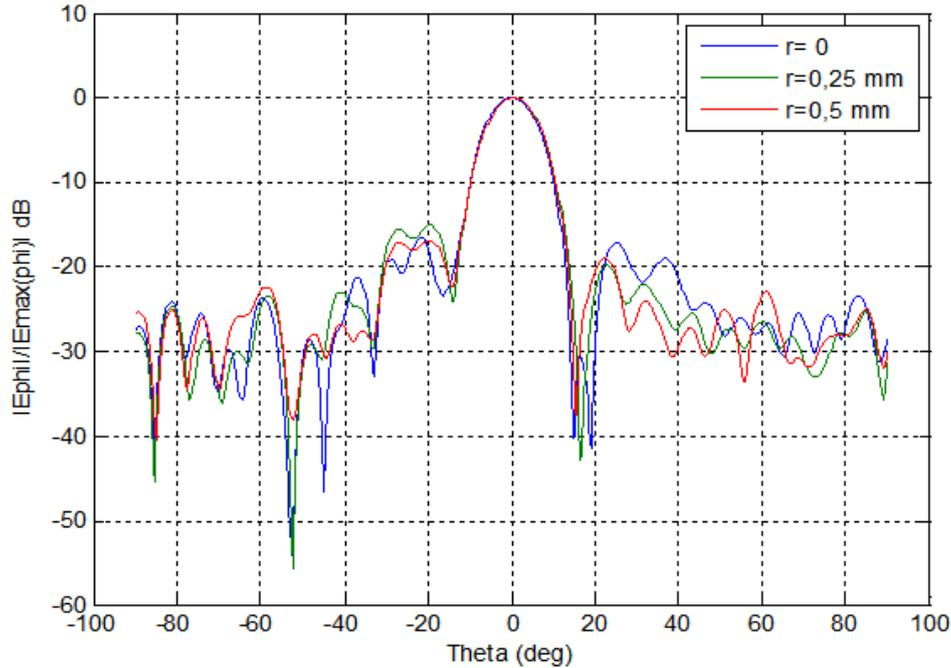
Figure 4: Radiation patterns of the E-plane at  $F=80$  GHz,  $b=0.8\lambda_0$  ;  $l=2.5$  mm;  $w=0.3387\lambda_0$  ;  $B=8\lambda_0$  ;  $\Delta y = \Delta z=1.0667\lambda_0$  ; 6 range of 7 slots.
