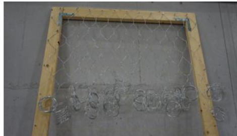
Figure 8: The gabion wire mesh produced manually by the second author
