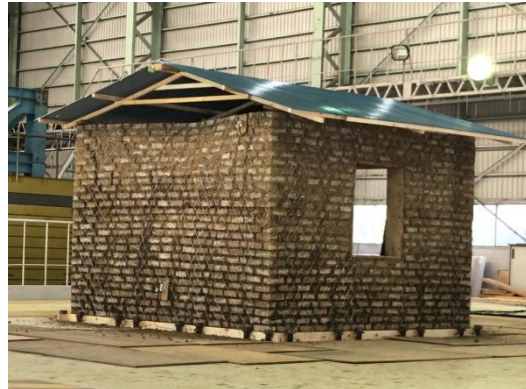
Figure 17: June 4, 2019 shaking table test with 50% JMA Kobe (left) and 70% JMA Kobe (right) input motion for Model B only
