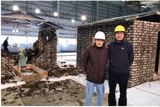
Figure 18: February 26, 2019 shaking table test: Model A collapsed & Model B still standing due to 70% JMA Kobe
