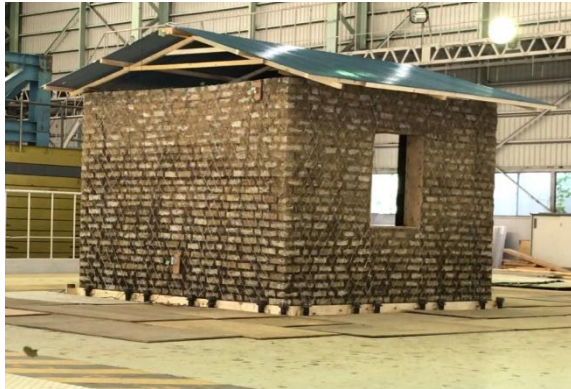
Figure 17: June 4, 2019 shaking table test with 50% JMA Kobe (left) and 70% JMA Kobe (right) input motion for Model B only
