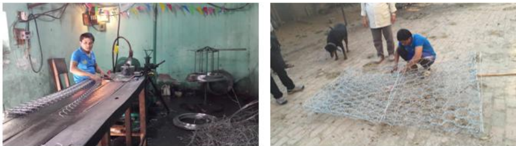
Figure 4: Gabion wire mesh produced in Nepal
