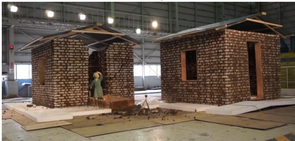
Model A (left) collapsed; Model B (right) survived
