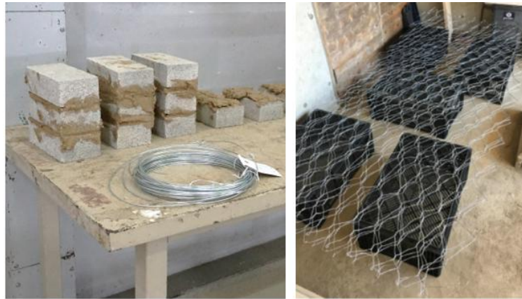
Figure 7: Materials used to construct mud mortar stone masonry
