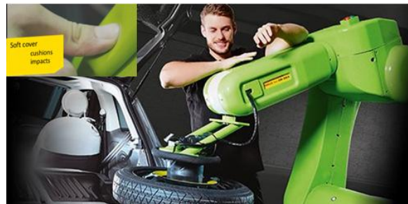
Figure 2: Collaborative robot sensitivity that causes the robot to stop [15]
