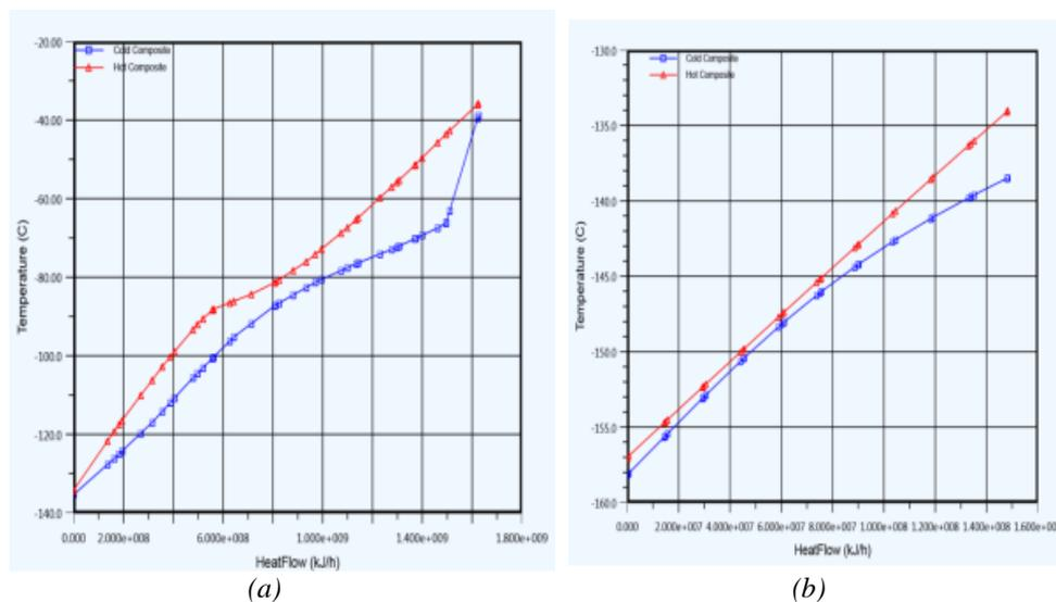
Figure 4: Temperature profiles showing the cold and hot composite curves for the Bottom (a) and Top (b) parts of the MCHE.
