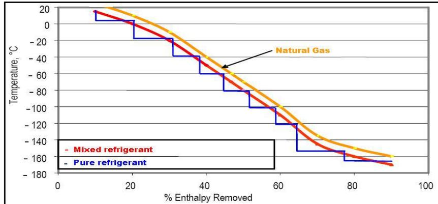
Figure 1: Cooling curves of pure refrigerant and mixed refrigerant (MR) versus NG [8]
