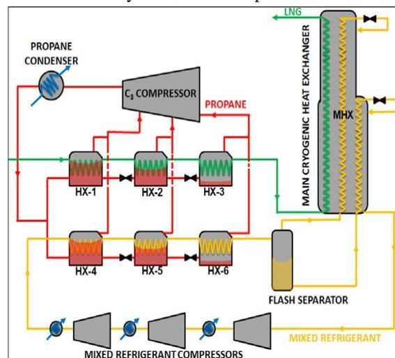
Figure 2: C3-MR process flow diagram [5]
