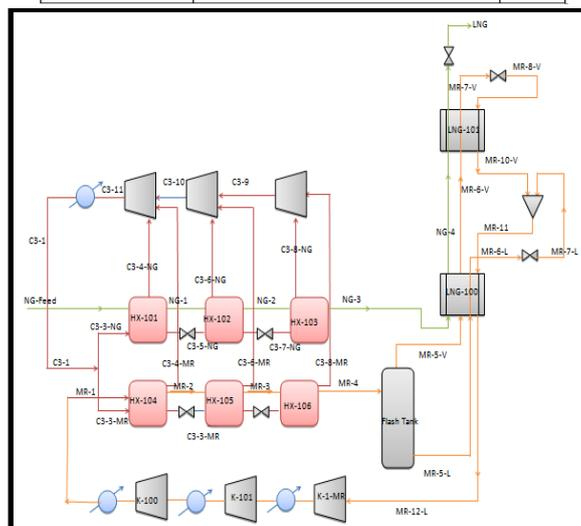
Figure 3: Process flow sheet of propane precooled mixed refrigerant cycle
