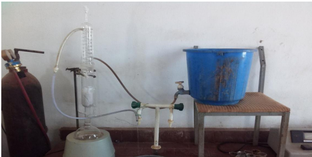
Figure 1: A set up for the calabash seed oil extraction unit (SERC)
