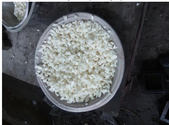
Figure 2: Polyurethane crushed as coarse aggregates
