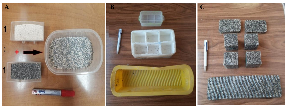
Figure 3: Photographs showing the steps of artificial ornamental stone production (A: Mixing of the two limestone waste samples together then with epoxy/resin, B: various molds and casting, C: the produced artificial ornamental stones)
