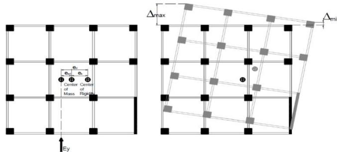
Figure 3: Calculation of maximum and minimum displacements
