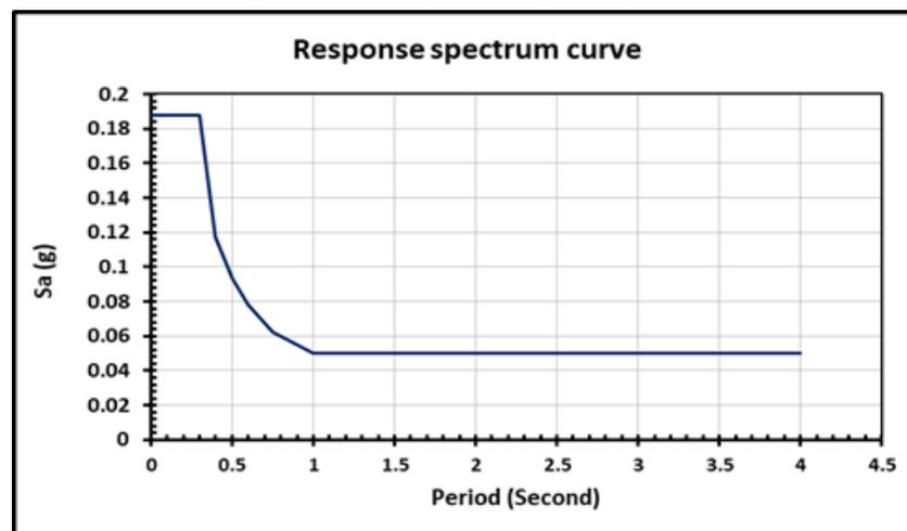
Figure 7: Response spectrum curve
