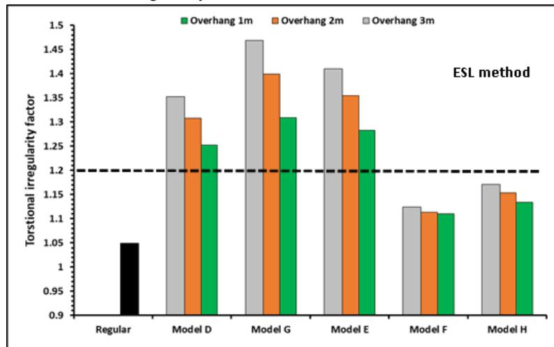
Figure 8: Torsional irregularity factor for 6-story buildings in case of ESL method
