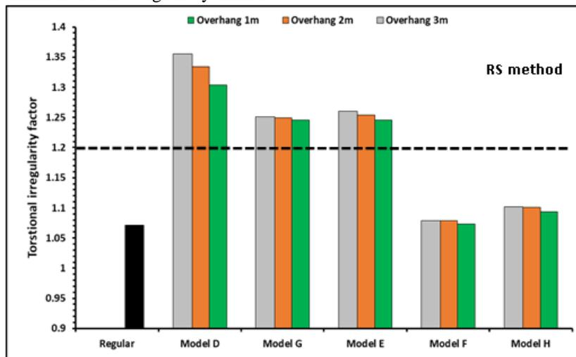
Figure 11: Torsional irregularity factor for 9-story buildings in case of RS method
