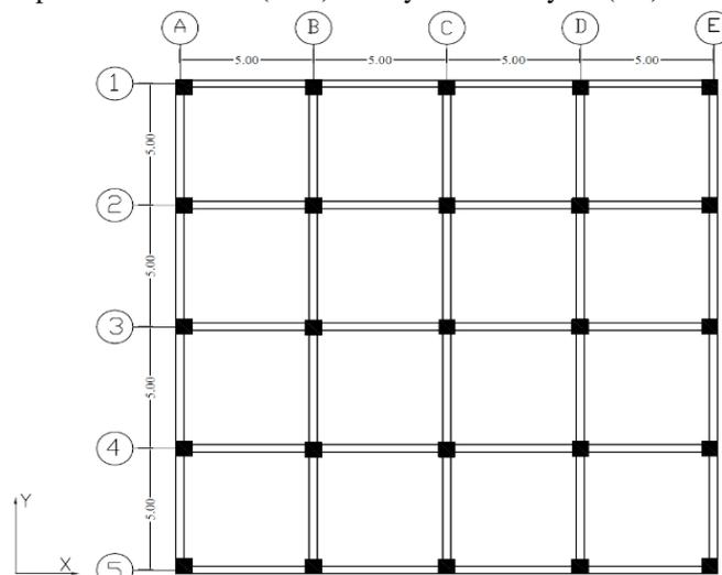
Figure 4: Plan of reference Model (Regular)
