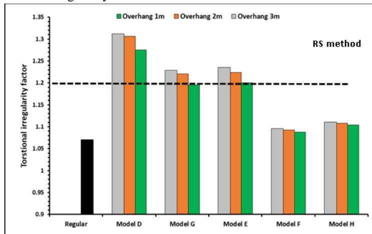
Figure 9: Torsional irregularity factor for 6-story buildings in case of RS method
