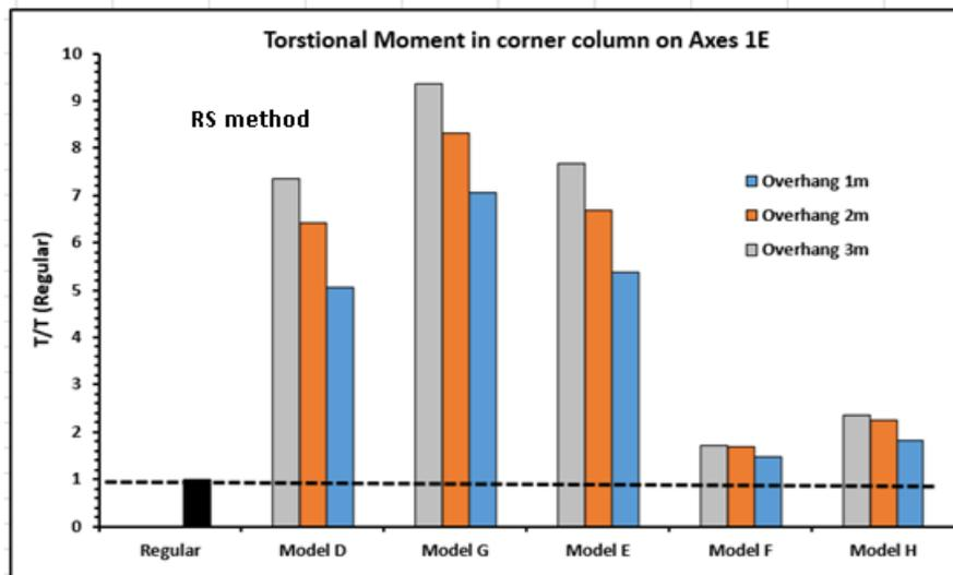
Figure 13: Torsional moment ratios for 6-story buildings with respect to the regular model in case of RS method
