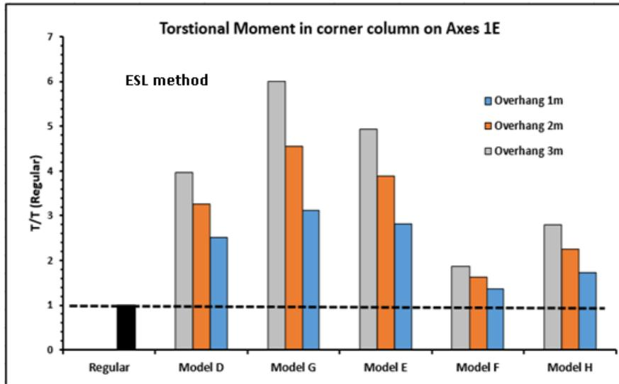
Figure 12: Torsional moment ratios for 6-story buildings with respect to the regular model in case of ESL method
