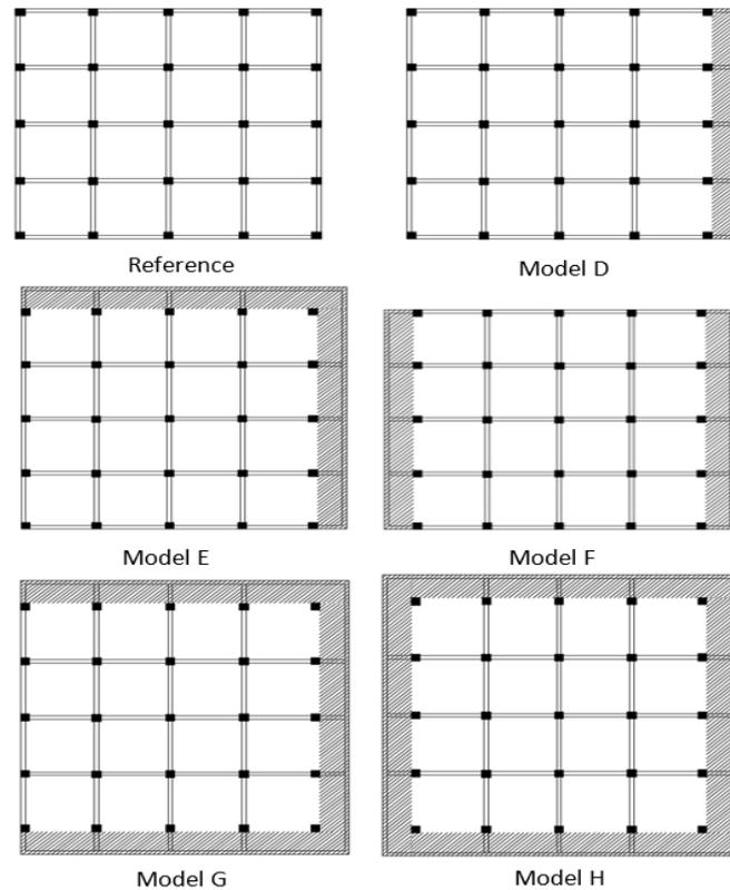
Figure 5: Plan view of building models
