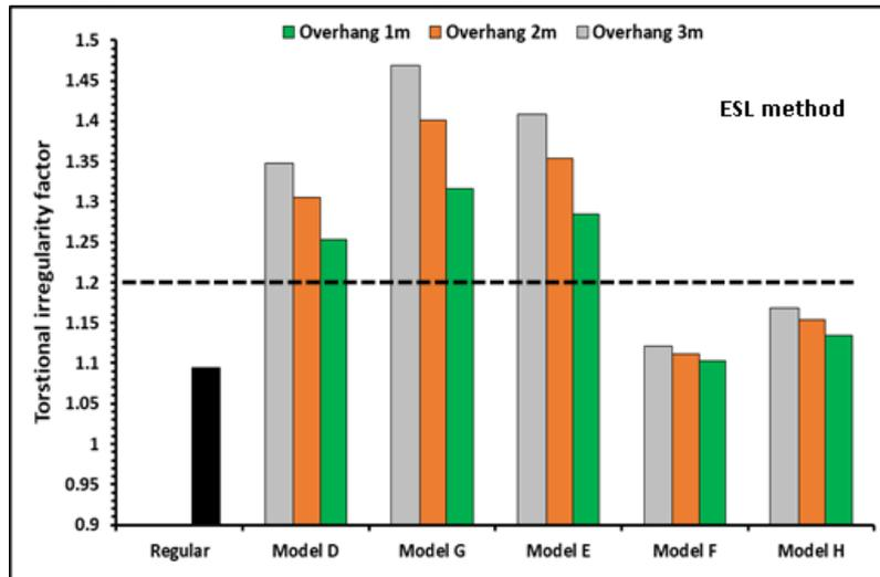
Figure 10: Torsional irregularity factor for 9-story buildings in case of ESL method
