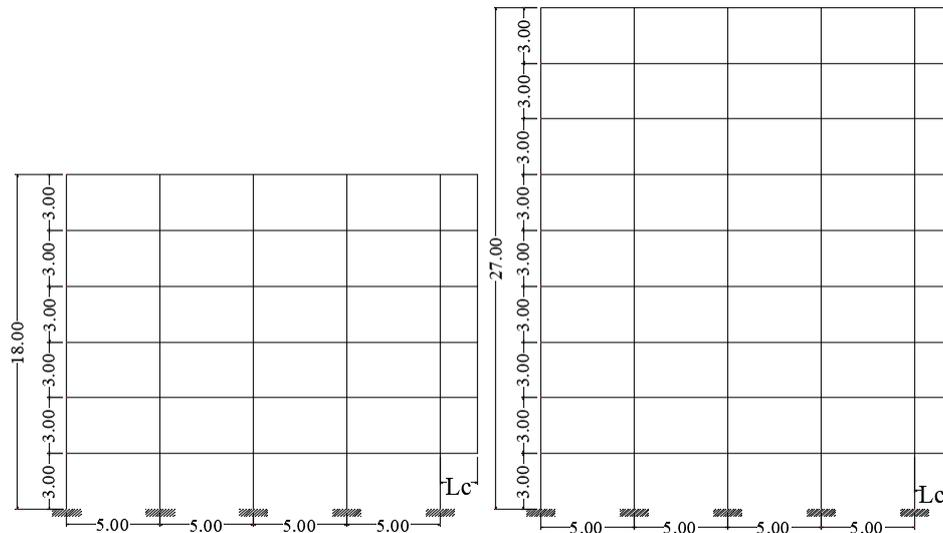
Figure 6: Elevation view of 6- and 9-story model D
