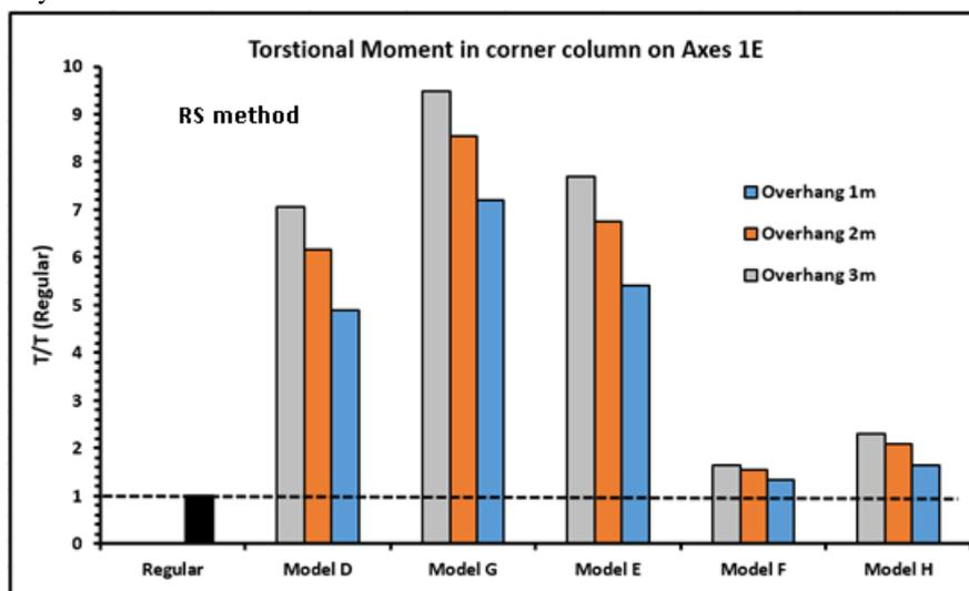
Figure 15: Torsional moment ratios for 9-story buildings with respect to the regular model in case of RS method
