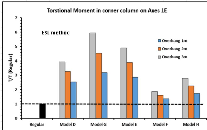
Figure 14: Torsional moment ratios for 9-story buildings with respect to the regular model in case of ESL method
