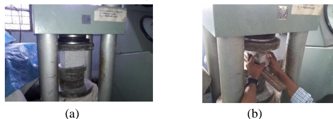
Figure 5: Measurement of (a) Compressive strength and (b) Splitting tensile strength
