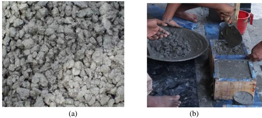
Figure 3: (a) After mixing the all ingredients (b) Making the sample block
