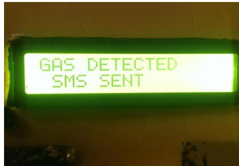
Figure 10: Gas leakage Condition of the Project after the message is sent
