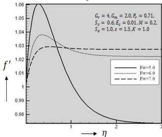
Figure 8: Primary velocity profiles for different values of  $f_w$
