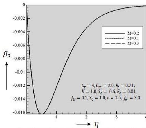
Figure 14: Secondary velocity profiles for different values of  $M$
