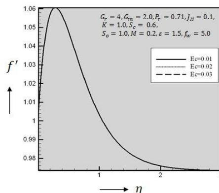
Figure 3: Primary velocity profiles for different values of  $E_c$
