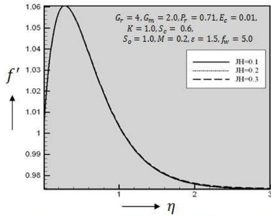
Figure 4: Primary velocity profiles for different values of  $J_H$
