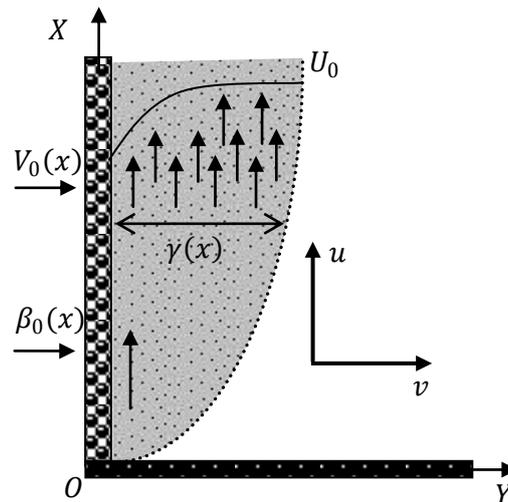
Figure 1: Geometrical configuration of boundary layer and coordinate system
