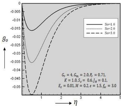
Figure 12: Secondary velocity profiles for different values of  $S_o$
