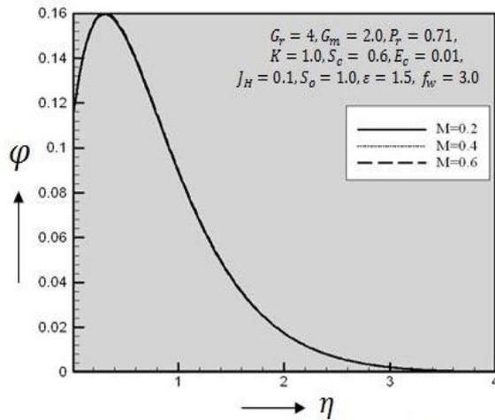
Figure 28: Concentration profiles for different values of  $M$
