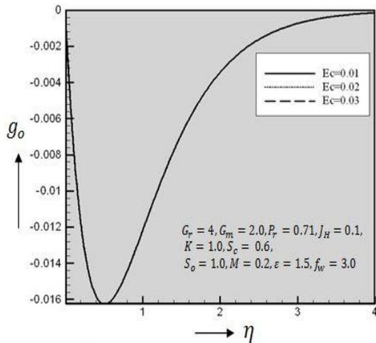
Figure 10: Secondary velocity profiles for different values of  $E_c$
