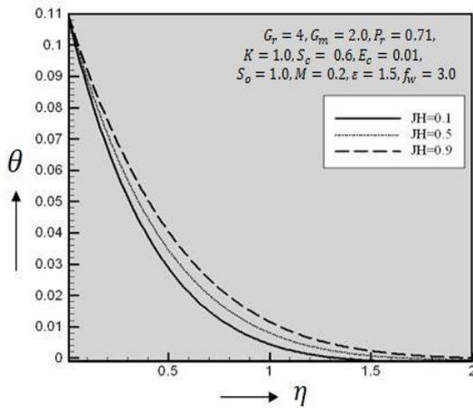
Figure 18: Temperature profiles for different values of  $J_H$
