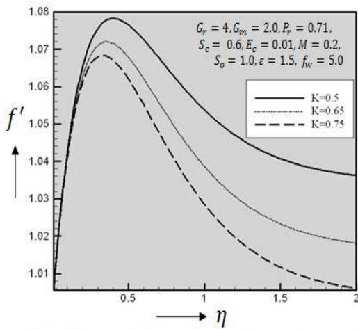
Figure 6: Primary velocity profiles for different values of  $K$
