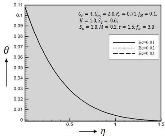
Figure 17: Temperature profiles for different values of  $E_c$
