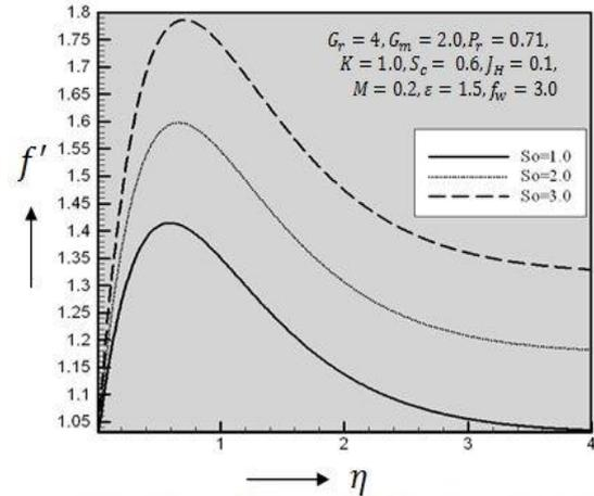
Figure 5: Primary velocity profiles for different values of  $S_o$
