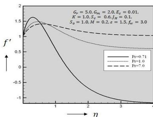
Figure 2: Primary velocity profiles for different values of  $Pr$
