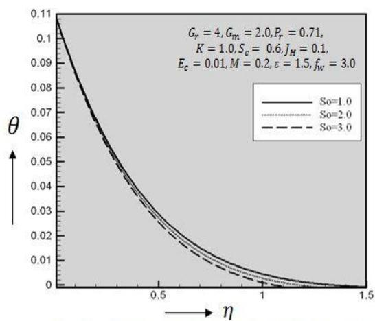
Figure 19: Temperature profiles for different values of  $S_o$
