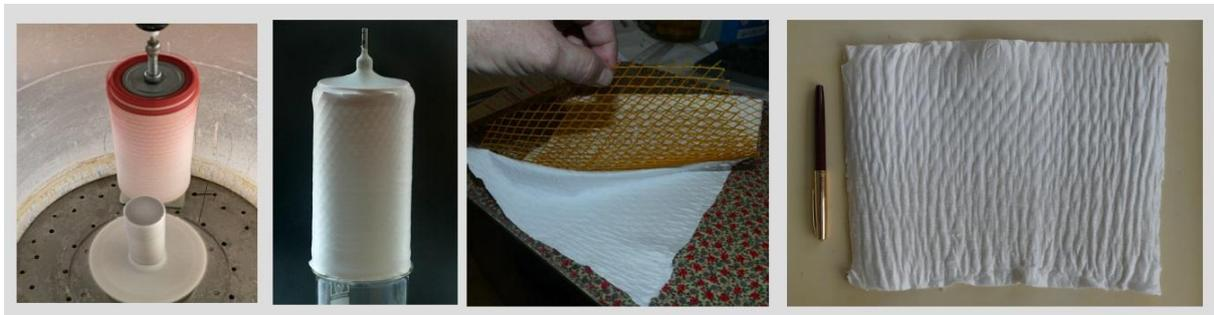
Figure 2: Preparation of the PHB submicron fiber mat by the centrifugal spinning technology and a rotating fiber collector
