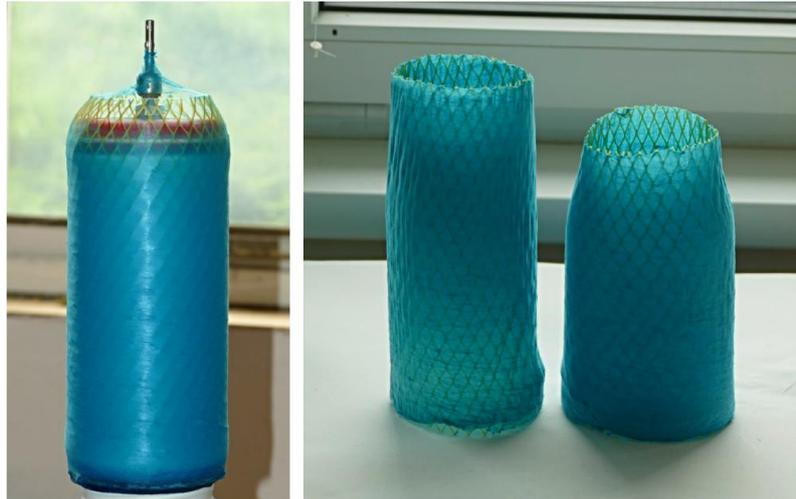
Figure 7: The PHB submicron fiber mats, loaded with the Zn phthalocyanine derivative, prepared by the centrifugal spinning technology using the rotating fiber collector
