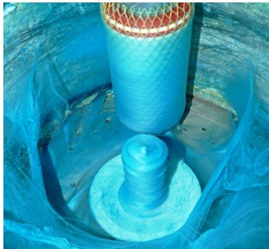
Figure 3: Preparation of the PHB submicron fiber mat and cobweb like structures, loaded with the Zn phthalocyanine derivative, by the centrifugal spinning technology and a rotating fiber collector
