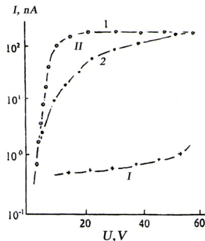
Figure 2: Photo (II) and dark (I) current-voltage characteristics of vidicon targets based on  $a - Si : H$ : 1-boron-doped sample, 2-undoped sample.
