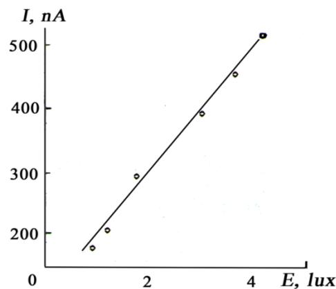
Figure 1: Luxampere characteristic of vidicon targets based on a - Si:H.
