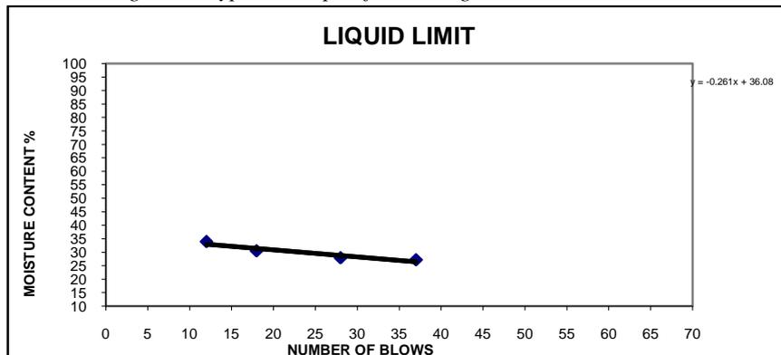
Figure 6: Typical Graph of Atterberg Limit at CH 20 + 500
