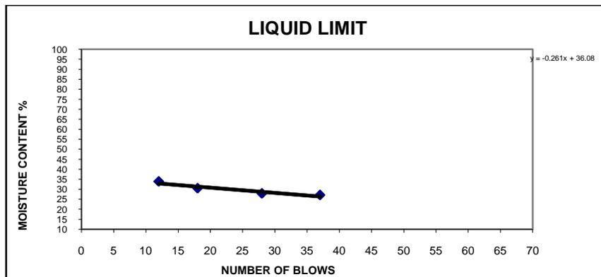
Figure 5: Typical Graph of Atterberg Limit at CH 10 + 500
