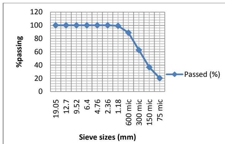
Figure 3: Typical Graphs of Sieve sizes Vs % passing at CH 10 + 500
