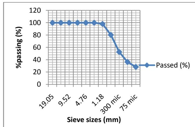
Figure 4: Typical Graphs of Sieve sizes Vs % passing at CH 20 + 500
