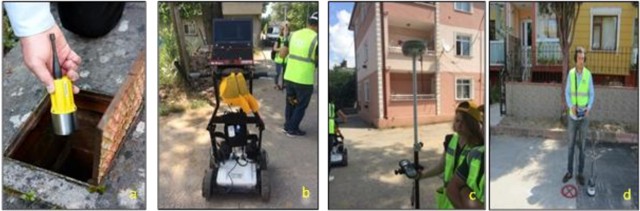
Figure 8: Permalog (a), GPR (b), GPS (c) and Acoustic Sonar Microphone (d)
