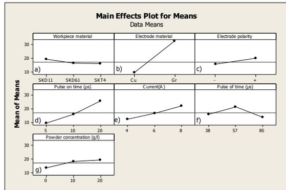
Figure 1: Main effects plot for  $\overline{MRR}$
