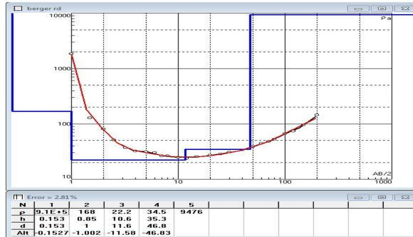
Figure 11: Apparent Resistivity versus Half-Current Electrode Spacing Curve for Berger Road
