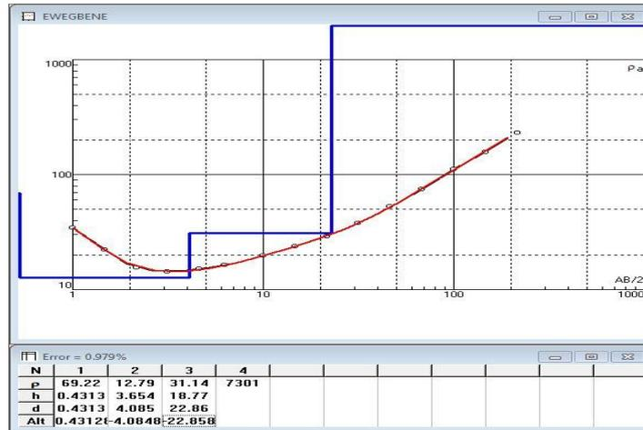
Figure 4: Apparent Resistivity versus Half-Current Electrode Spacing Curve for Ewegbene
