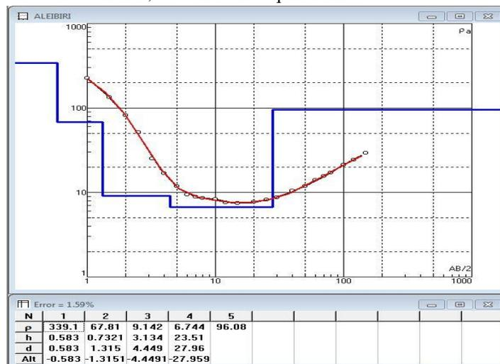
Figure 3: Apparent Resistivity versus Half-Current Electrode Spacing Curve for Aleibiri 1
