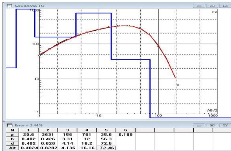
Figure 6: Apparent Resistivity versus Half-Current Electrode Spacing Curve for Sagbama 1
