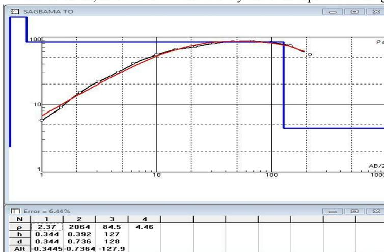
Figure 7: Apparent Resistivity versus Half-Current Electrode Spacing Curve for Sagbama 2
