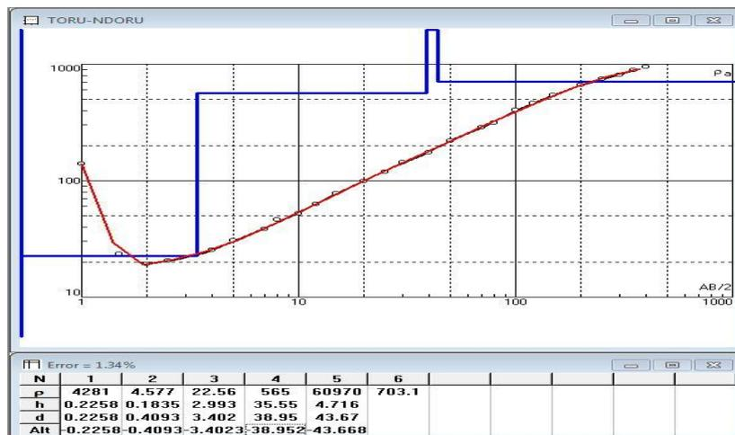
Figure 10: Apparent Resistivity versus Half-Current Electrode Spacing Curve for Toru Ndoru
