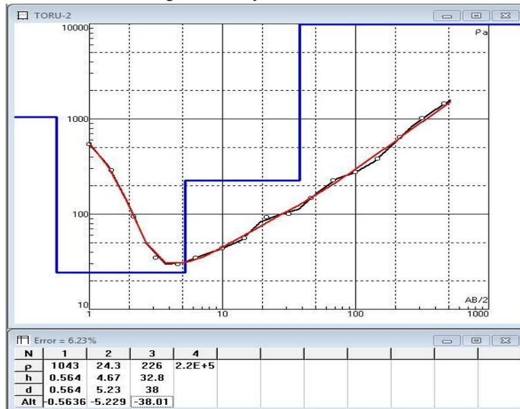
Figure 9: Apparent Resistivity versus Half-Current Electrode Spacing Curve for Toru 2
