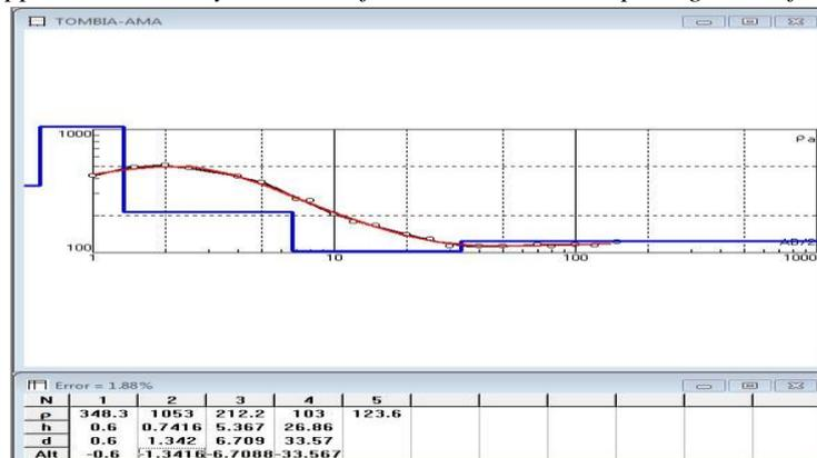
Figure 8: Apparent Resistivity versus Half-Current Electrode Spacing Curve for Tombia-Ama
