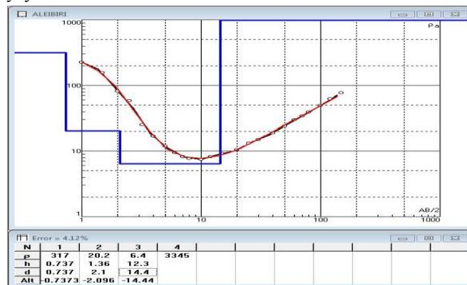
Figure 2: Apparent Resistivity versus Half-Current Electrode Spacing Curve for Aleibiri
