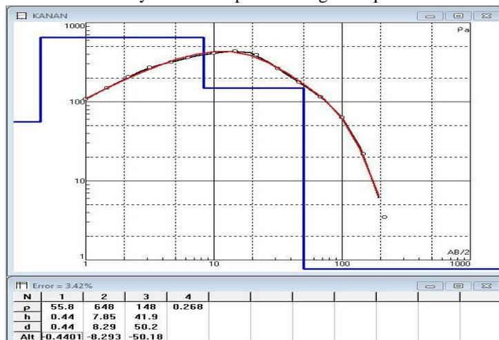
Figure 5: Apparent Resistivity versus Half-Current Electrode Spacing Curve for Kanan
