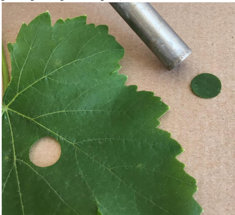
Figure 3: Taking samples with a special circular punch 1.50 cm in diameter from the left and right sides of the veins along the main veins of the leaf
