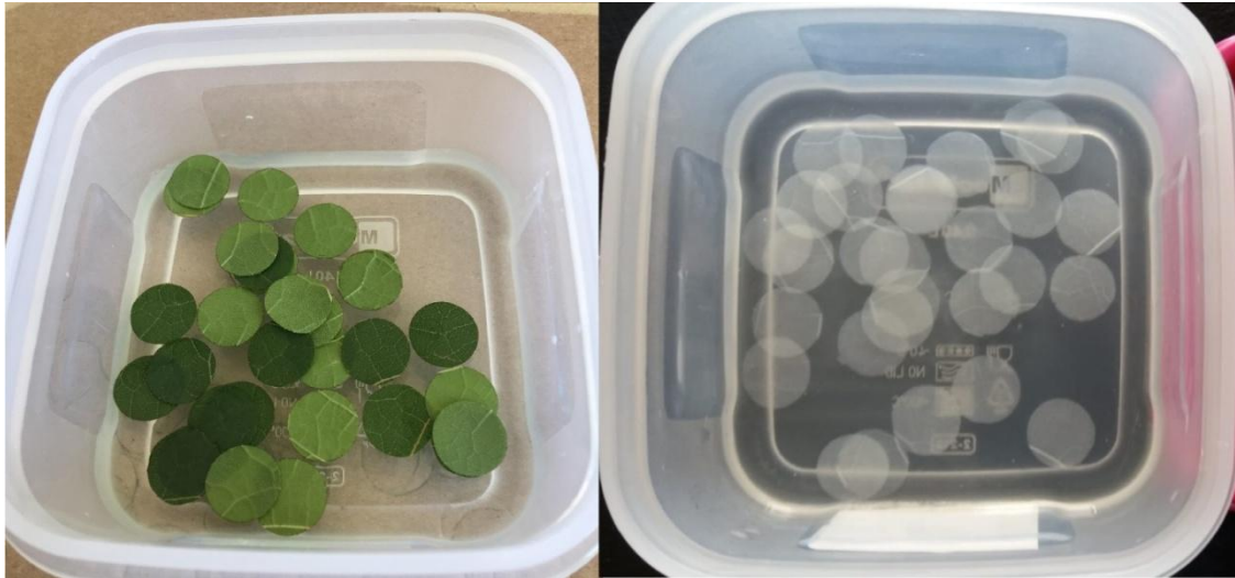
Figure 4: Placing circular green leaf samples in Sodium hypochlorite (2.5%) solution (left). After circular leaf samples kept at room temperature (22-23 °C) for 10-12 hours, are completely transparent (right)
