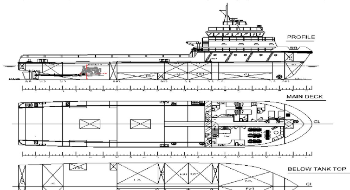
Figure 1: Depiction of Offshore Servicing Vessel in Two Different Views
