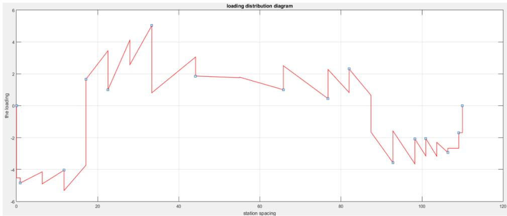
Figure 13: Light Ship net load Curve
