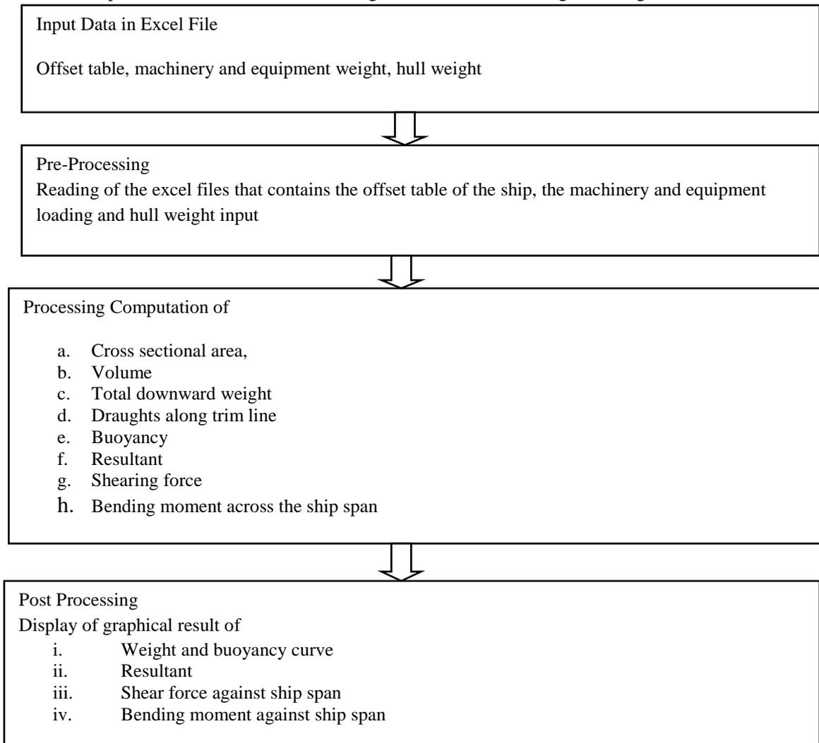
Figure 5: Block Diagram for Developing Shear Force and Bending Moment Matlab Programmed
