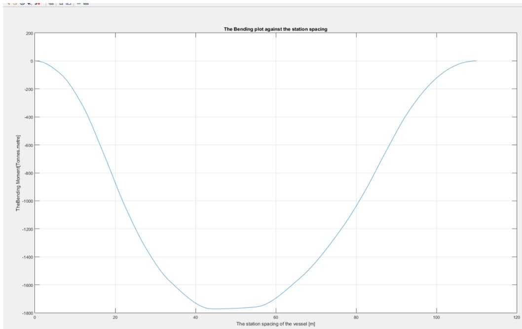
Figure 15: Light Ship Bending Moment Diagram
