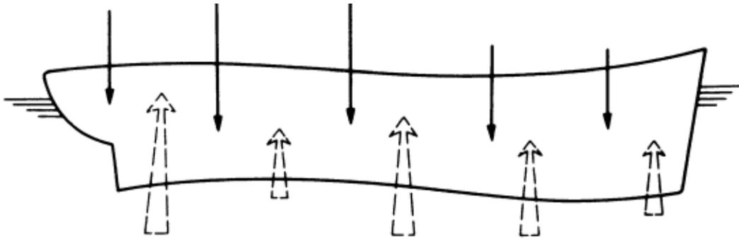
Figure 2: Action of gravity and buoyant loadings on a hull structure [3]
