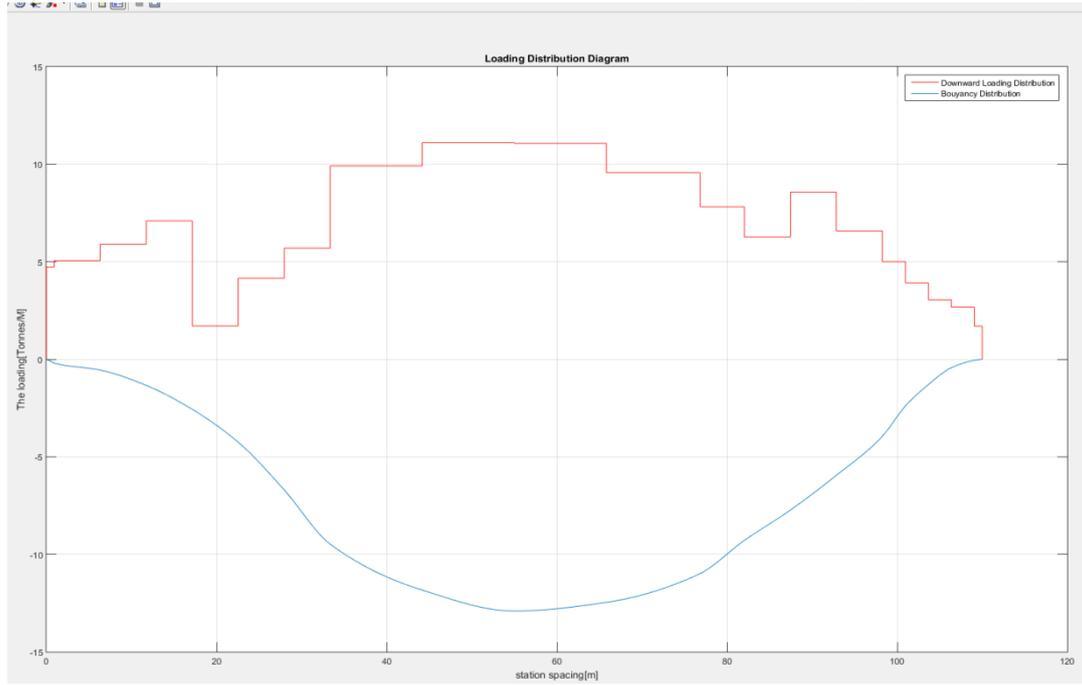
Figure 12: Light Ship Weight and Buoyancy Distribution curves
