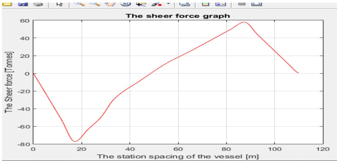
Figure 14: The Graph of the Light Ship Shear Forces
