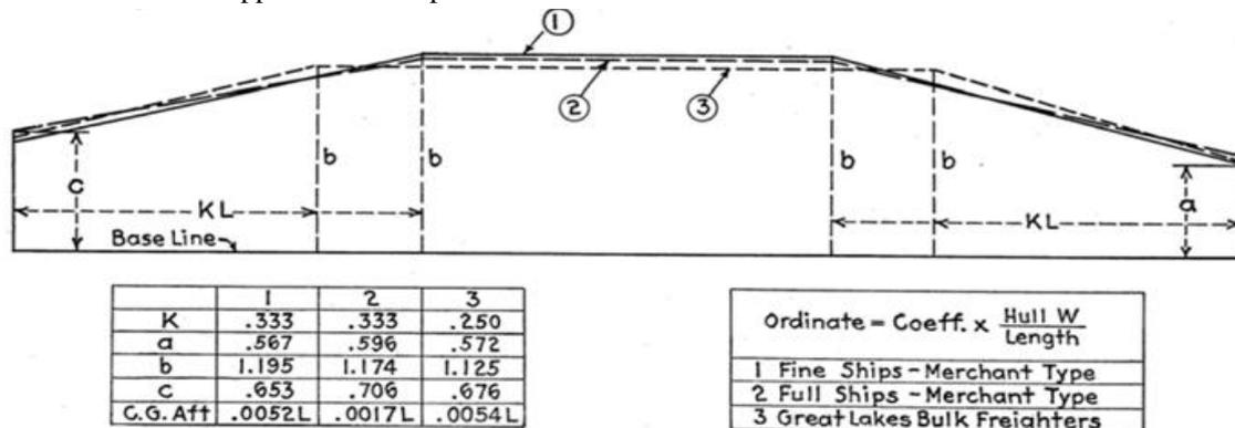
Figure 4: Approximation to Hull Weight of Mid Parallel Body
