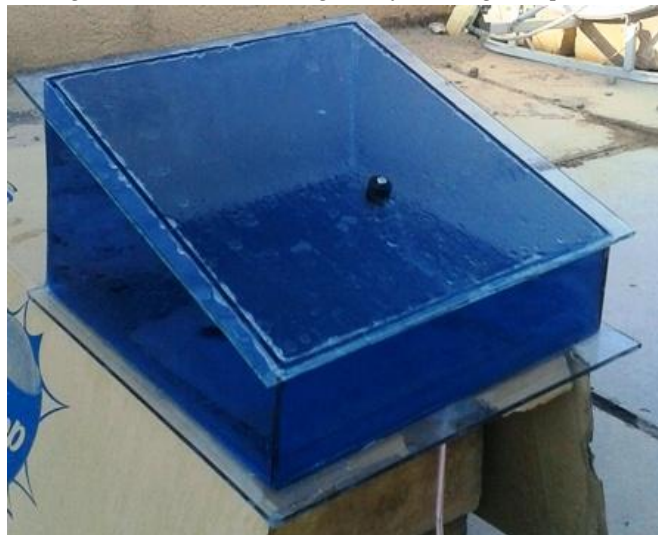
Figure 2b: A photographic picture of the Single Slope Solar Still (glass one face reflector)
