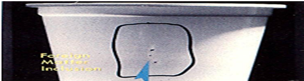
Figure 12: A picture of a Foreign Matter Inclusion
