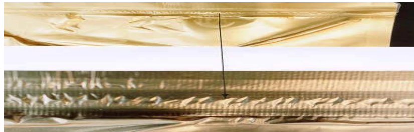
Figure 30: Blister defect in flexible film materials
