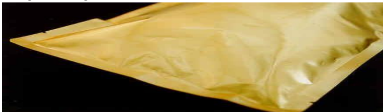
Figure 35: picture of a swollen defect
