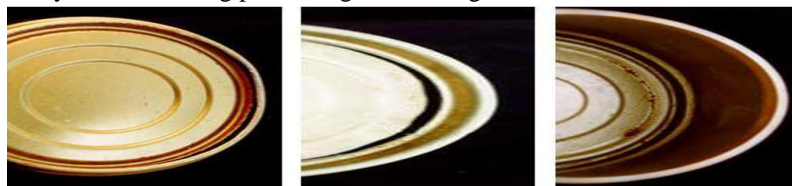
Figure 24: Fractured Bottom Profile
