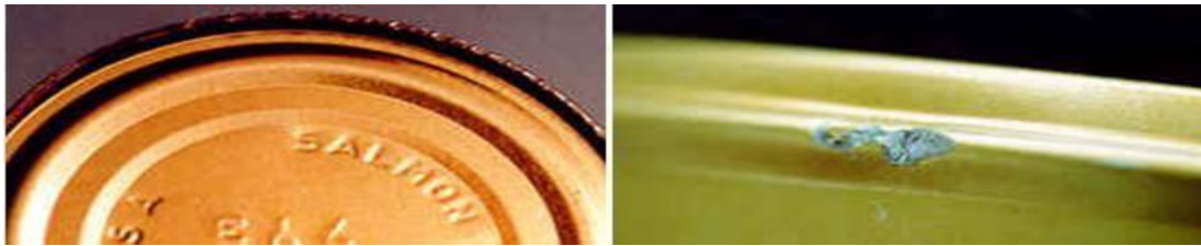
Figure 27: Abrasion defect in metals
