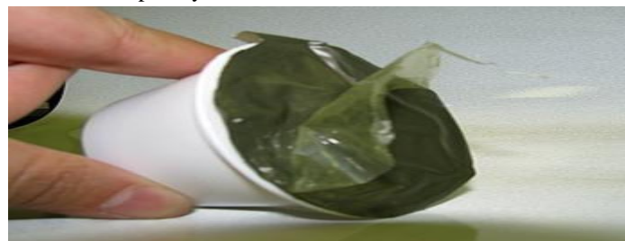
Figure 10: A picture of a Cut (fracture) defect
