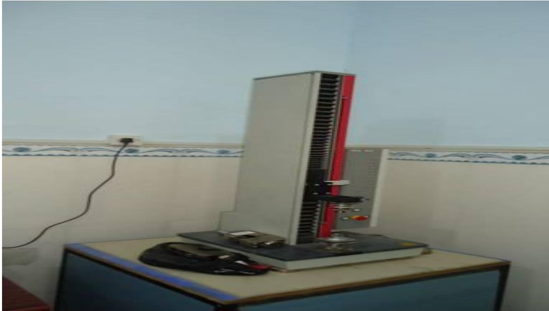
Figure 3: Tensile test of the specimens was carried out with a Zwick/Roel type [BT1-FR2.5 TN.D14]
