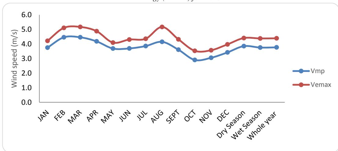
Figure 11: Plot showing the variation of the most probable wind speed ( $V_{mp}$ ) and the wind speed carrying maximum energy ( $V_{emax}$ ) for Ijebu-ode.
