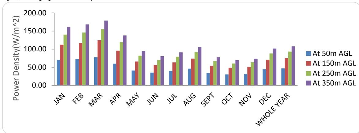
Figure 12: Monthly variation of power densities for the extrapolated mean wind speeds for Abeokuta
