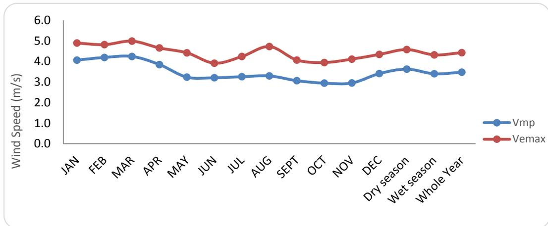
Figure 10: Plot showing the variation of the most probable wind speed ( $V_{mp}$ ) and the wind speed carrying maximum energy ( $V_{emax}$ ) for Abeokuta.
