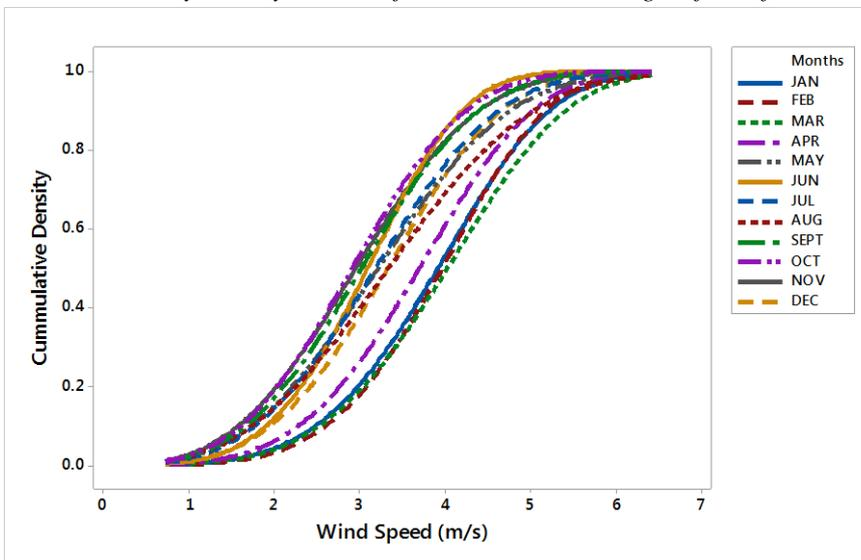
Figure 7: Cumulative Distribution Function for whole years at Height of 10m for Abeokuta.
