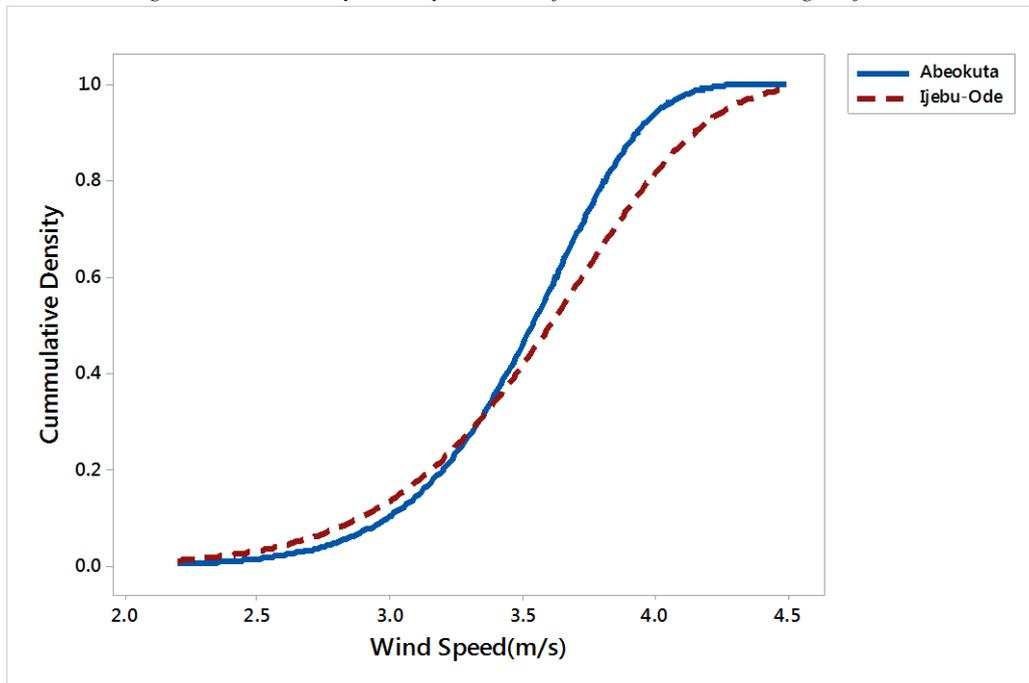
Figure 5: Cumulative Distribution Function for whole years at Height of 10m
