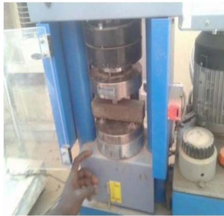
Figure 5 : Flexion tests machine of 250 KN class 1
