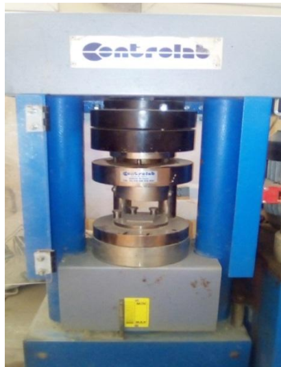
Figure 6 : Compression tests machine of 250 KN class 1
