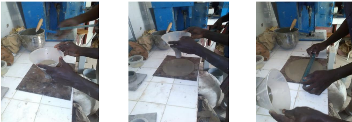
Figure 4 : Checking of the sand concrete spreading
