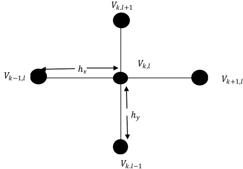
Figure 1: Five Point Stencil for Potential Computation
