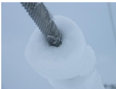
Figure 1: The iced conductor
