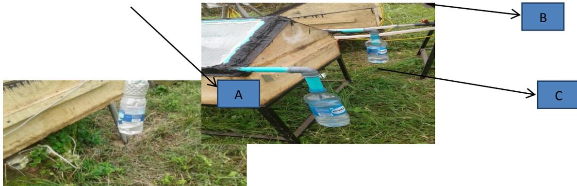
Plate 2: Distillate output (A,B,C) for single slope and double slope solar still
