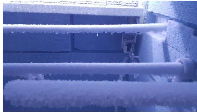
Figure 3: The iced conductor in ACC
